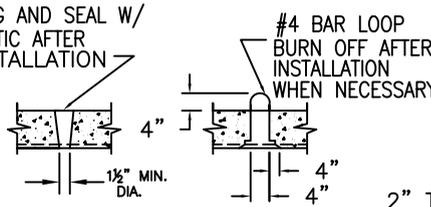
**WELDED WIRE FABRIC REINFORCEMENT**
