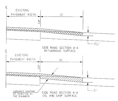
IF EXISTING SUB-BASE IS INADEQUATE, AS DETERMINED BY THE ENGINEER, THE SIDEROADS SHALL BE CORED OUT AND AGGREGATE SUB-BASE, TYPE B SHALL BE PLACED FOR THE BASE. THE COST OF CORING OUT THE SIDEROAD SHALL BE INCLUDED IN THE COST OF THE AGGREGATE BASE COURSE. IF EXISTING SUB-BASE IS DETERMINED TO BE ADEQUATE, THE AGGREGATE BASE COURSE SHALL BE DELETED AND THE PREPARATION OF THE BASE SHALL BE CONSTRUCTED ACCORDING TO ARTICLE 406.19.
