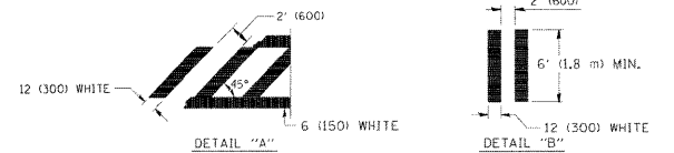
TYPICAL CROSSWALK MARKING
