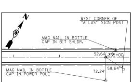
\*95530 STA 280+00.00 (MAG NAIL) IN BOTTLE CAP IN PWR POLE (MAG NAIL) IN BOTTLE CAP ON BIT. SHLDR. WEST COR OF "ATLAS" SIGN
