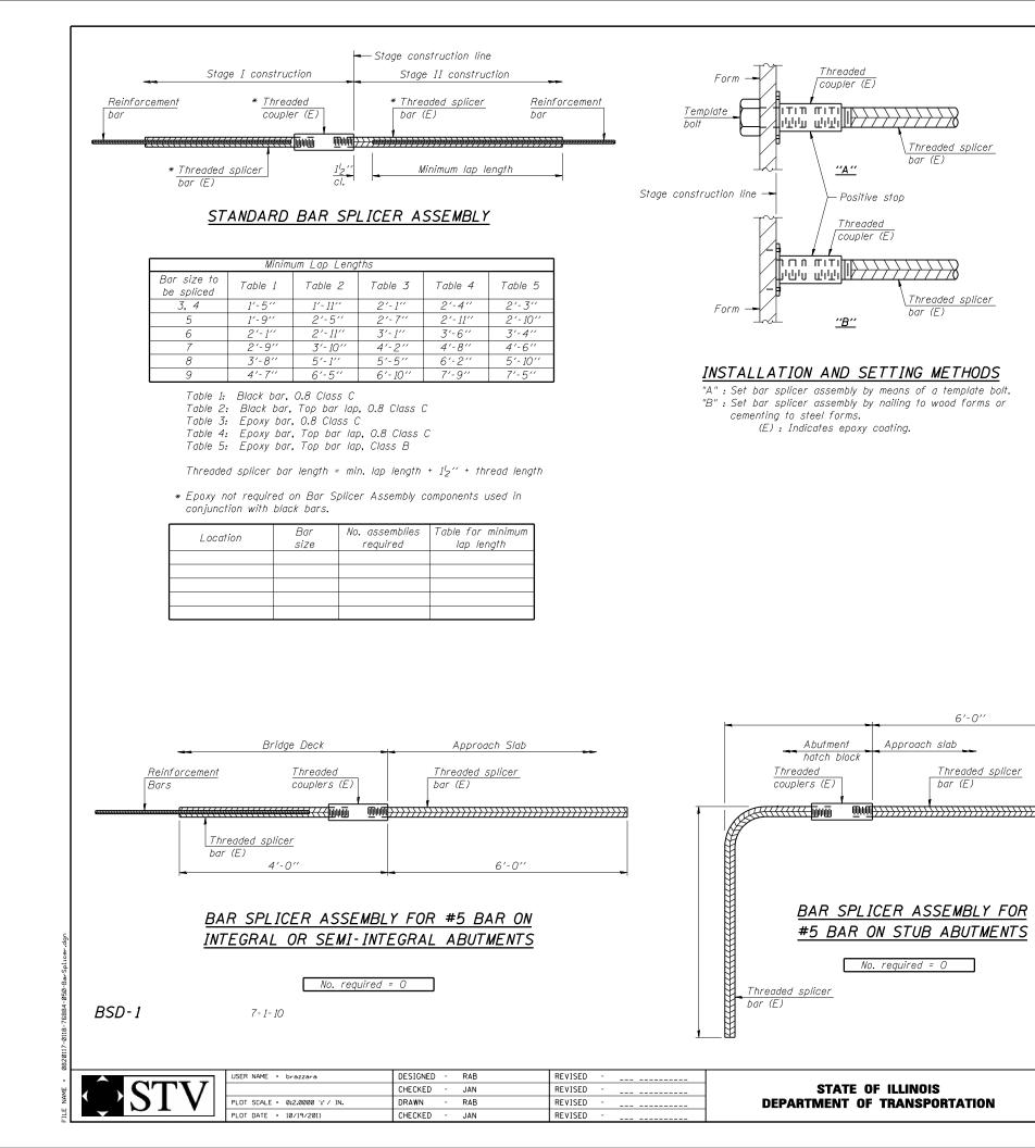
BAR SPLICER ASSEMBLY AND MER STRUCTURE NO. 082-0117 (E.I. SHEET NO. S-50 OF S
