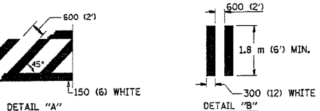
TYPICAL CROSSWALK MARKING
