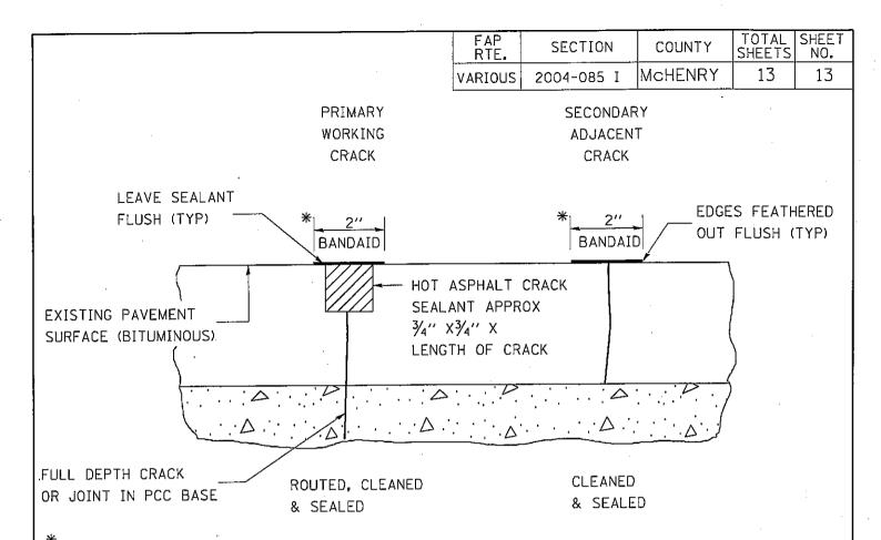
IN ALL LOCATIONS WHERE THE LONGITUDINAL CRACK CONFLICTS WITH EXISTING PAVEMENT MARKINGS (EITHER EDGE LINE OR LANE LINE) THE CRACK SHALL BE ROUTED & THE RESULTING RESERVOIR FILLED WITH SEALANT. HOWEVER, THE 2" BANDAID SEALANT STRIP SHALL BE DELETED TO PREVENT UNNECESSARY DAMAGE TO THE EXISTING PAVEMENT MARKINGS. ALL DAMAGES TO EXISTING PAVEMENT MARKINGS & RAISED REFLECTIVE PAVEMENT MARKERS IN EXCESS OF THAT CAUSED BY THE ROUTING OPERATION SHALL BE REPLACED AT THE EXPENSE OF THE CONTRACTOR.
