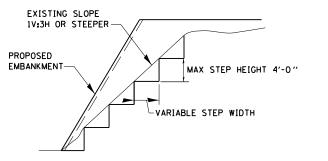
EXISTING 19:3H OR STEEPER SLOPES SHALL BE STEPPED PRIOR TO PLACING NEW EMBANKMENT.
