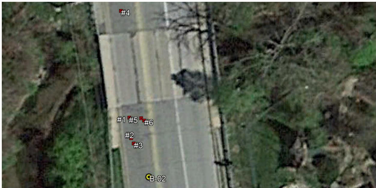
Exhibit #1) Plan view showing attempted drill locations (#1 to #6) and final boring location B-02.
