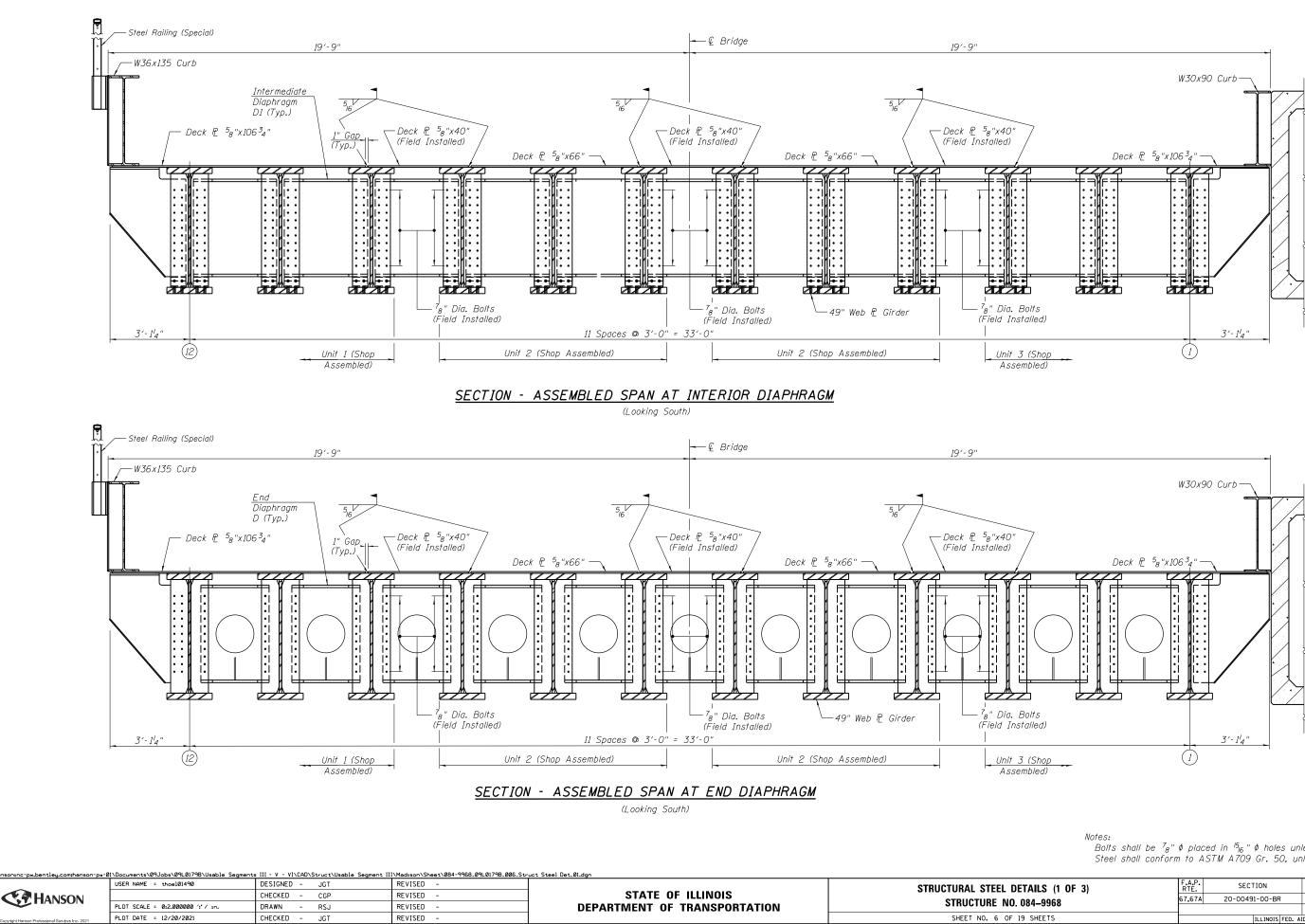
Bolts shall be  $7_8$ "  $\phi$  placed in  $^{15}_{6}$ "  $\phi$  holes unless otherwise noted. Steel shall conform to ASTM A709 Gr. 50, unless otherwise noted.
