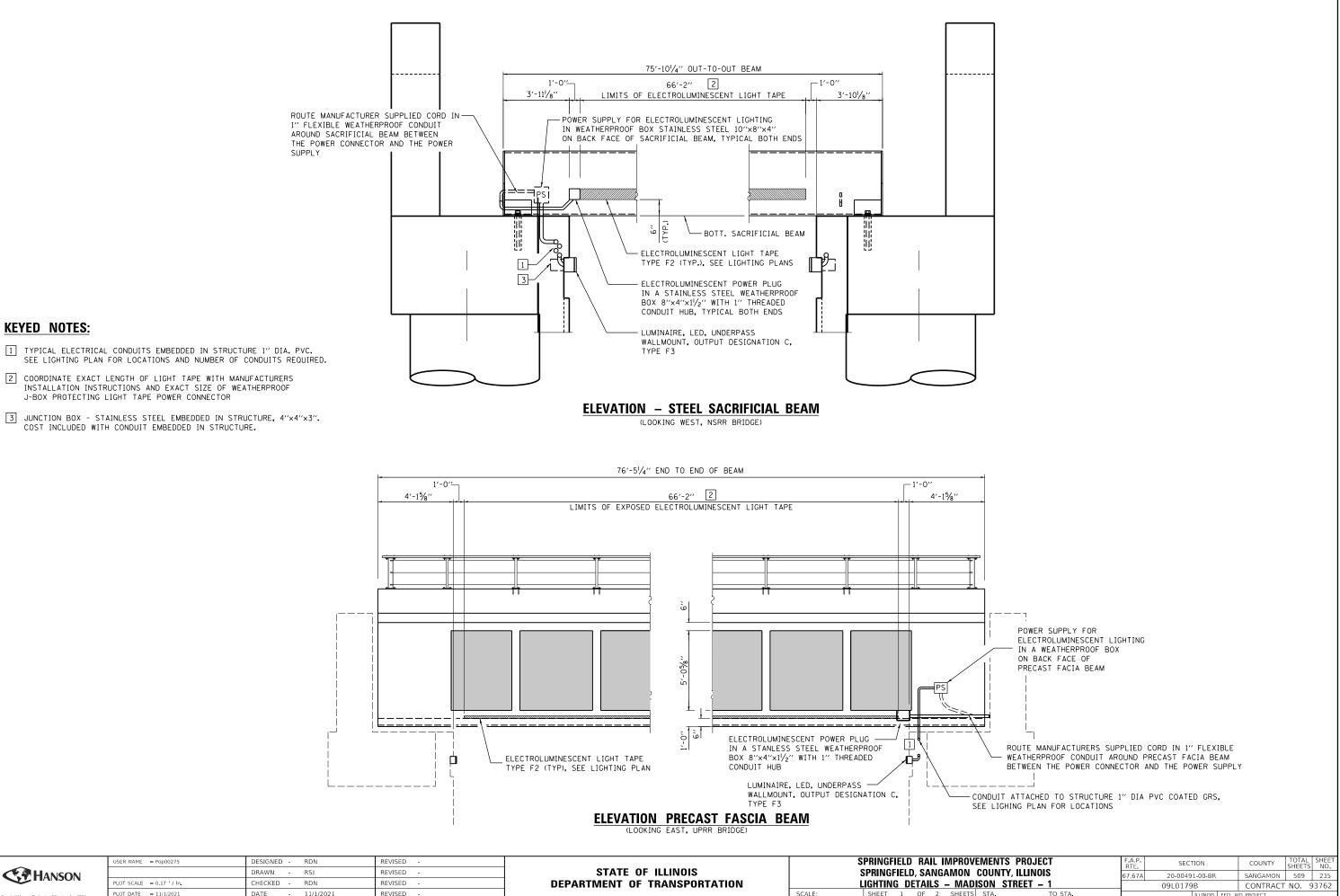
3 JUNCTION BOX - STAINLESS STEEL EMBEDDED IN STRUCTURE, 4"×4"×3".
