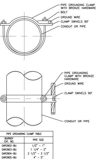
PIPE GROUNDING CLAMPS SHALL HAVE BRONZE HARDWARE, BE CORROSION RESISTANT, SUITABLE FOR DIRECT BURIAL IN EARTH OR CONCRETE. & UL467 LISTED.
