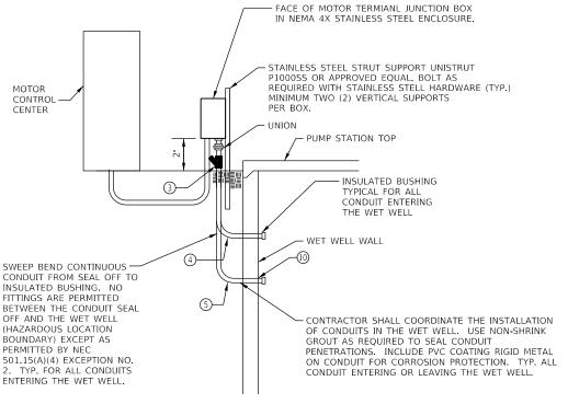
CONDUIT FROM SEAL OFF TO INSULATED BUSHING. NO FITTINGS ARE PERMITTED BETWEEN THE CONDUIT SEAL OFF AND THE WET WELL (HAZARDOUS LOCATION BOUNDARY) EXCEPT AS PERMITTED BY NEC. 501.15(A)(4) EXCEPTION NO. 2. TYP. FOR ALL CONDUITS ENTERING THE WET WELL.
