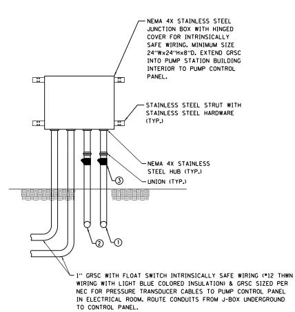
1 INTRINSICALLY SAFE JUNCTION BOX ELEVATION
