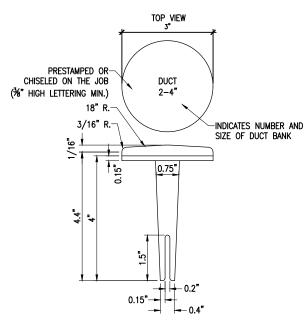
BITUMINOUS PAVEMENT DUCT MARKERS "NOT TO SCALE"
