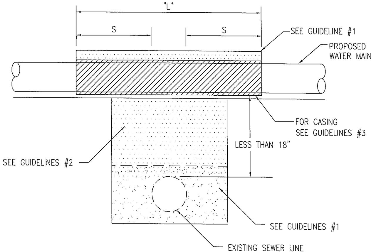
NOTE: "S" THE LENGTH NECESSARY TO PROVIDE 10 FEET OF SEPARATION AS MEASURED PERPENDICULAR TO THE EXISTING SEWER LINE.
