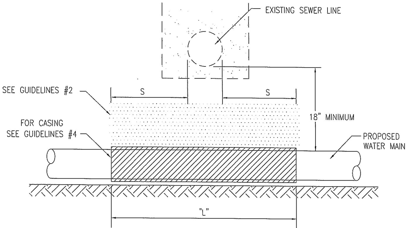
NOTE: "S" THE LENGTH NECESSARY TO PROVIDE 10 FEET OF SEPARATION AS MEASURED PERPENDICULAR TO THE EXISTING SEWER LINE
