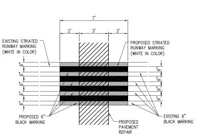
PROPOSED PAVEMENT REPAIR AND STRIATED CENTERLINE MARKING DETAIL "NOT TO SCALE"
