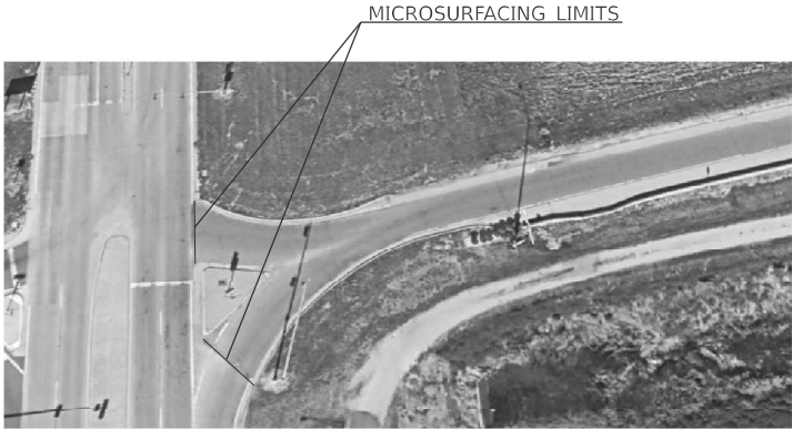
MICROSURFACING LIMITS AT COLLINSVILLE RD.
