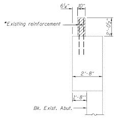
\* Existing reinforcement extending into the area of new approach slab construction shall be cleaned, straightened and incorporated into the new construction. Any reinforcement bars being reused that are damaged during concrete removal operations shall be repaired or replaced using an approved bar splicer or anchorage system. Cost included in Concrete Removal.
