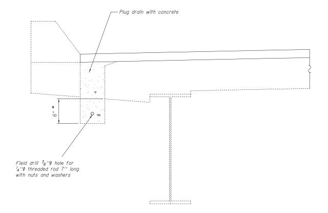
\*Cut off drain 6" below the deck
