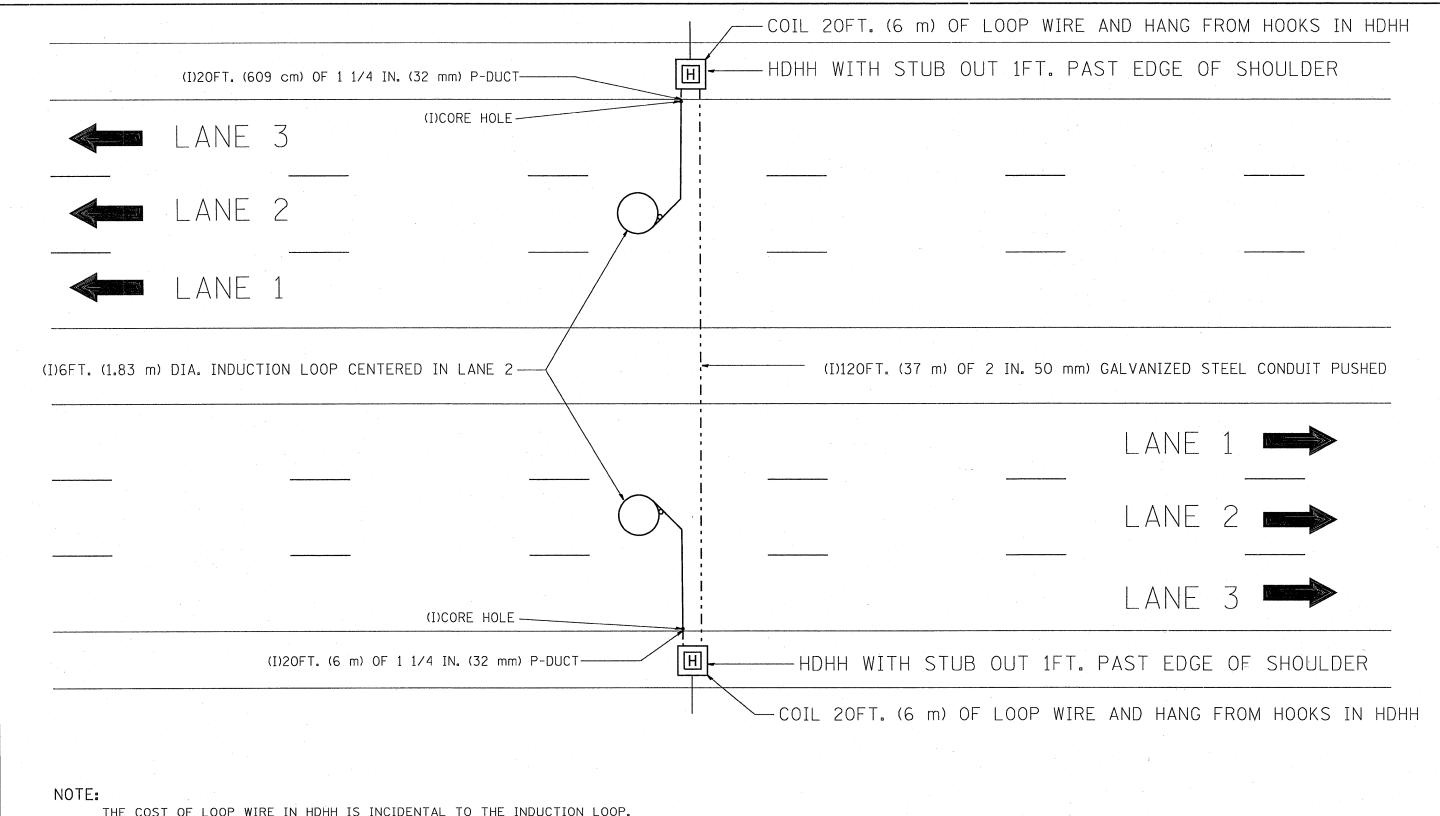
THE COST OF LOOP WIRE IN HOHH IS INCIDENTAL TO THE INDUCTION LOOP. IT SHALL NOT BE MEASURE FOR PAYMENT.
