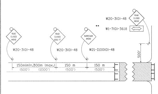
ROAD CLOSED TO THRU TRAFFIC BARRICADE SET UP
