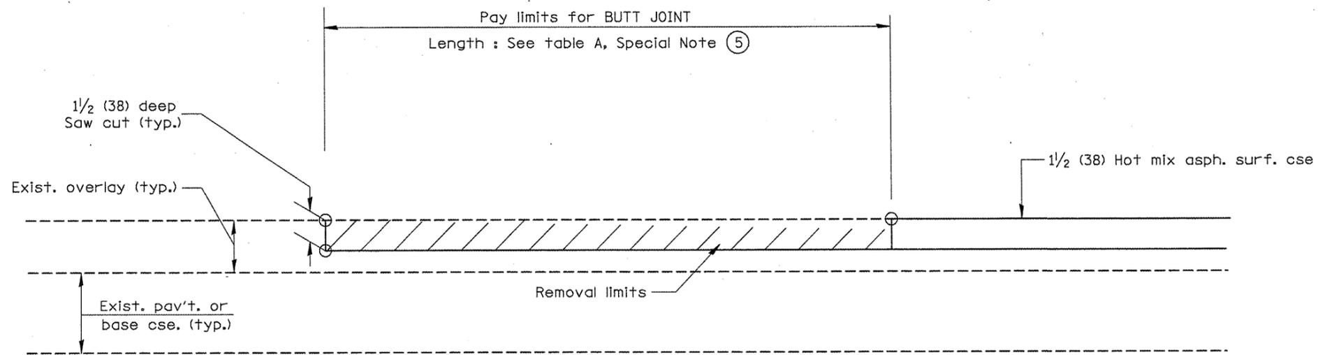
CASE 5 : WITH HOT MIX ASPHALT SURFACE REMOVAL (COLD MILLING)
