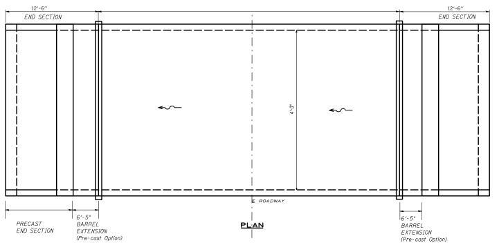
The Precast end section and pre-cast barrel extensions are paid for as BOX CULVERT END SECTION, CULVERT NO. 2 (EACH).
