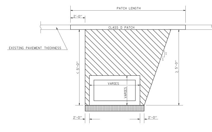
PAY LIMITS OF POROUS GRANULAR EMBANKMENT - CA-6 UNLESS OTHERWISE SHOWN IN DETAILS
