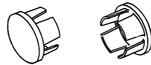
CAST END CAP DRIVE FIT TYPE 8- Required Incidental to item "Aluminum Handrail".
