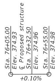
US 45 PROFILE GRADE (Along centerline roadway)
