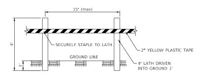
MATERIALS ARE TO BE APPROVED BY ENGINEER PRIOR TO INSTALLATION. COST OF MATERICAL, INSTALLATION, RELOCATION AND MAINTENANCE OF LATHING AND WARNING TAPE IS TO BE INCIDENTAL TO ITEM A5150530 TRAFFIC MAINTENANCE.
