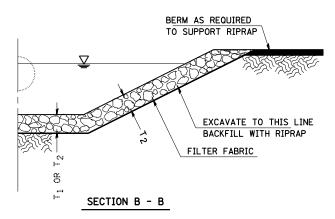
NOTE A - TRANSITION BASIN TO CONFORM TO THE NATURAL STREAM CHANNEL. TOP OF RIPRAP IN THE FLOOR OF THE BASIN SHOULD BE AT THE SAME ELEVATION OR LOWER THAN THE NATURAL CHANNEL BOTTOM AT SECTION " & SECTION ".
