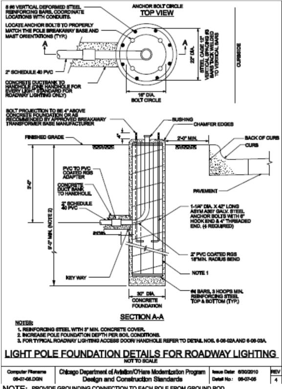
PROVIDE GROUNDING CONNECTION TO EACH POLE FROM GROUND ROD OF NEAREST HANDHOLE WITH #8 AWG BARE COPPER CONDUCTOR. THIS WORK IS INCIDENTAL TO PAY ITEM "LIGHT POLE CONCRETE
