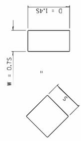
For diamond shaped sign with side S, as shown, use required post size for a sign with  $W = 0.75S$  and  $D = 1.45S$ .
