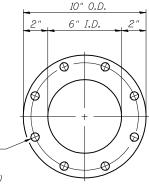
Drill and tap 8 holes for  $l_2$ "-13 bolts on an  $8^3_4$ "  $\phi$ bolt circle. (2 blind holes are  $l_4$ " deep, 6 thru holes)
