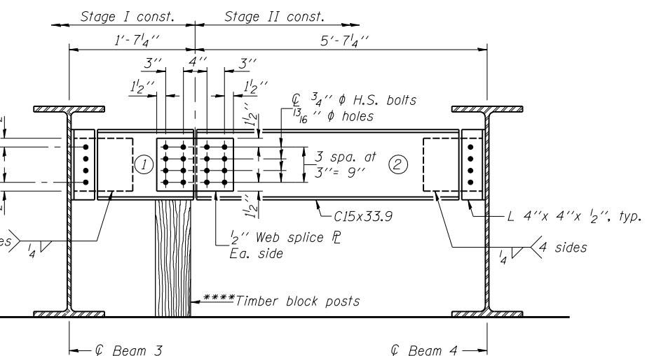
DIAPHARM D<sub>2</sub> AT STAGE CONSTRUCTION LINE
