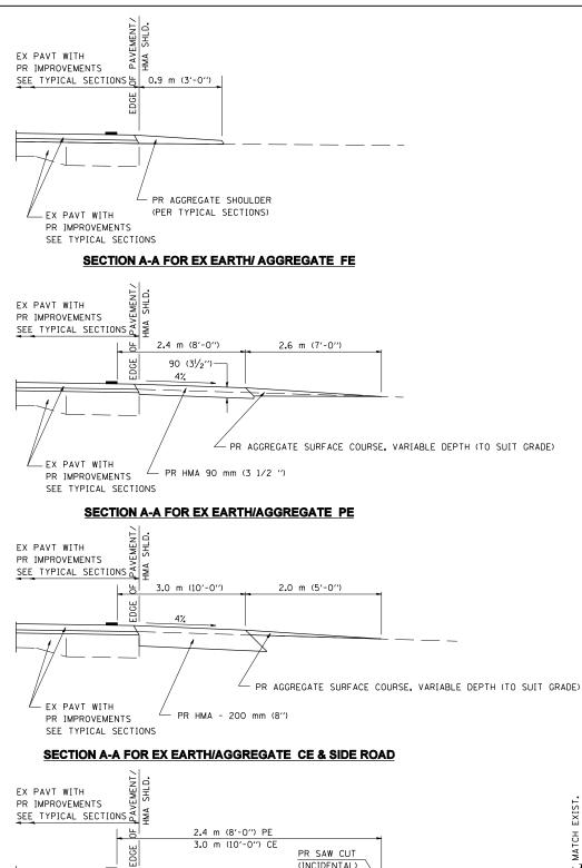
(INCIDENTAL) PR HMA SURFACE REMOVAL - BUTT JOINT (IF EXISTING HOT-MIX ASPHALT) PR PCC SURFACE REMOVAL - BUTT JOINT ( IF EXISTING PCC) EX PAVT WITH -PR HOT-MIX ASPHALT VAR DEPTH ± 38 mm (1 1/2 ") PR IMPROVEMENTS SEE TYPICAL SECTIONS 45°
