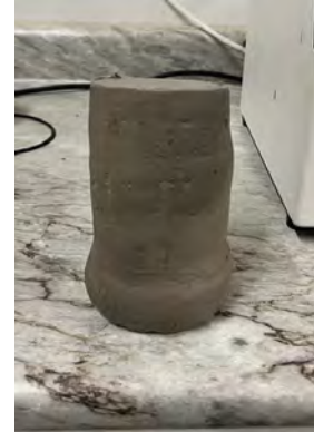
Failure Type: Bulge
