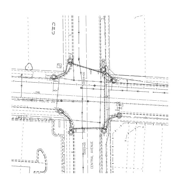
AT THE INTERSECTION OF US BUS 20 WITH CENTRAL AVE. THE FOLLOWING ITEMS SHALL BE INCLUDED AS, REMOVE EXISTING TRAFFIC SIGNAL EQUIPMENT AND REMAIN THE PROPERTY OF THE CITY OF ROCKFORD. CONTACT JEREMY CARTER, 1-815-967-6734, WITH CITY OF ROCKFORD FOR THE LOCATION OF DELIVERY OF THE REMOVED EQUIPMENT.
