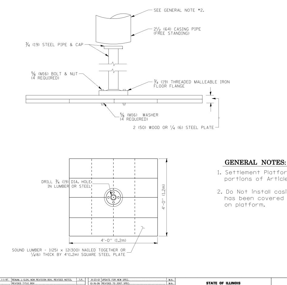
1. Settlement Platform shall be in accordance with the appicable portions of Article 204.06 of the Standard Specifications.
