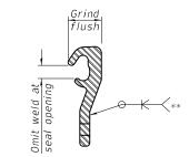
The strip seal shall be made continuous and shall have a minimum thickness of  $\frac{1}{4}$ ". The configuration of the strip seal shall match the configuration of the locking edge rails. Open or "webbed" strip seal gland configurations are not permitted. The gland shall be sized for a maximum
