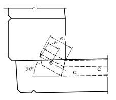
ELEVATION AT PARAPET (Skews ≤ 30°)
