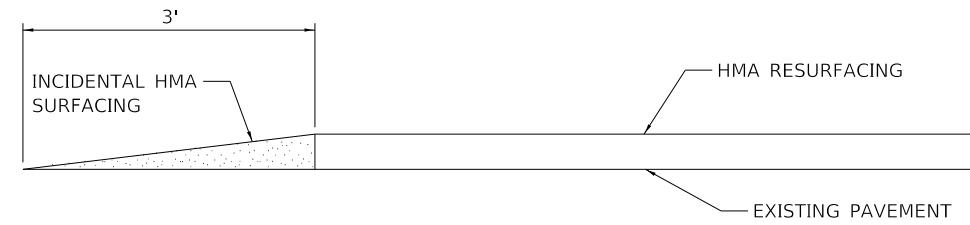
FEATHEREDGE DETAIL SECTION A-A
