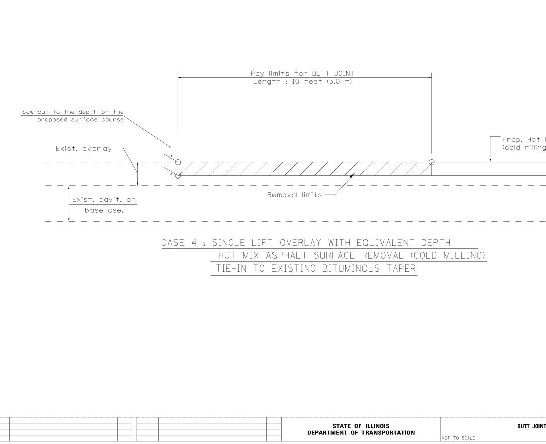
Prop. Hot Mix Asphalt surf. removal (cold milling) per plans.
