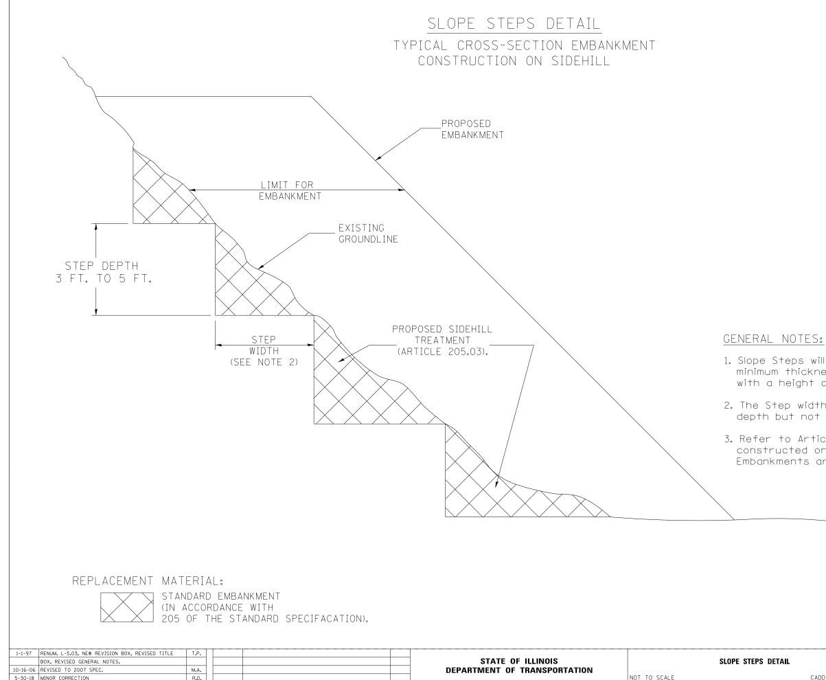
1. Slope Steps will be required for all 12(300) minimum thickness "sliver fills" and on all fills with a height of 10 feet or greater.
