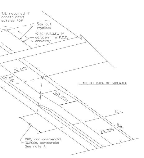
1. The sidewalk area located within the pay limits of P.C.C. Driveway Pavement will be of the same thickness and construction as the P.C.C. Driveway Pavement.
