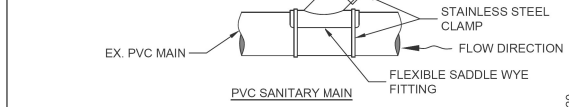
FLEXIBLE SADDLE CONNECTION DETAIL (FOR SERVICE CONNECTIONS TO PVC SANITARY MAINS LESS THAN 18" DIA.)
