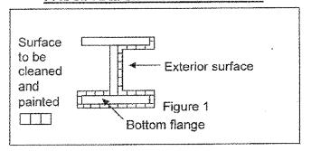
ALL BEAMS, BEARINGS AND OTHER STRUCTURAL STEEL WITHIN FIVE (5) FT., TEN (10) FT. AT LOCATION 4 (SN 056-0059), (MEASURED ALONG THE BEAM) OF EITHER SIDE OF THE DECK JOINTS INCLUDING JOINTS AT PIN & LINKS ON LOCATION 2 (SN 023-0106), SHALL BE CLEANED PER NEAR WHITE BLAST CLEANING SSPC-SP10. THE EXTERIOR SURFACES AND TOP AND BOTTOM OF THE BOTTOM FLANGE OF THE FASCIA BEAMS (SEE FIGURE 1) SHALL ALSO BE CLEANED PER NEAR WHITE BLAST CLEANING SSPC-SP10.
