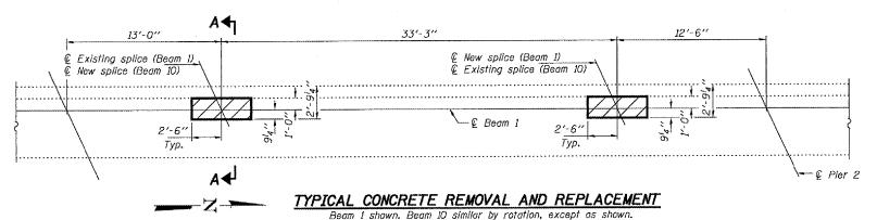
Hatched areas indicate concrete sections to be removed and replaced. Perimeters of concrete removal areas shall be saw cut <sup>3</sup>4" prior to the removal of concrete. Reinforcement shall be cut only if required for fitting bolts. Cut reinforcement shall be spilced as directed by the Engineer. Cost shall be included with Concrete Removal.
