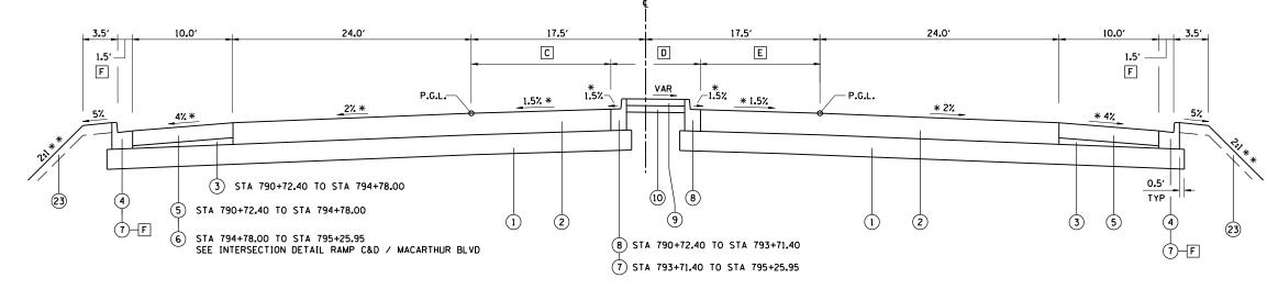
C STA 790+72.40 TO STA 793+84.40 = TAPER 24.0' TO 0.0' STA 793+84.40 TO STA 793+96.68 = 0.0' STA 793+96,68 TO STA 795+25,95 = VARIES SEE INTERSECTION DETAIL RAMP C&D / MACARTHUR BLVD
