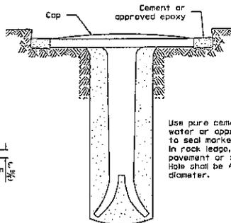
Tablet constructed in rock ledge or concrete.
