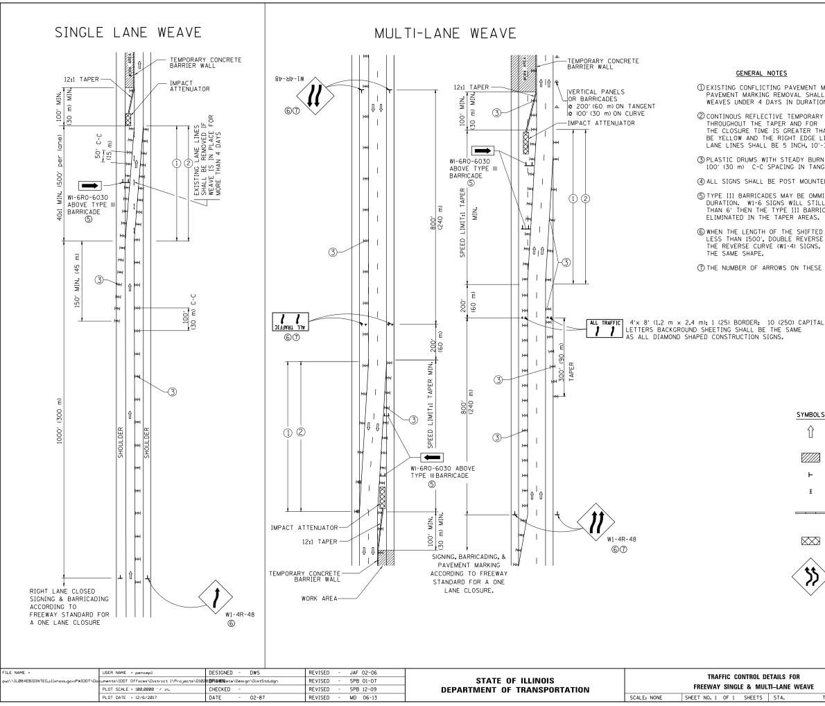
① EXISTING CONFLICTING PAVEMENT MARKING LINES SHALL BE REMOVED. PAVEMENT MARKING REMOVAL SHALL NOT BE REQUIRED FOR SINGLE LANE WEAVES UNDER 4 DAYS IN DURATION.
