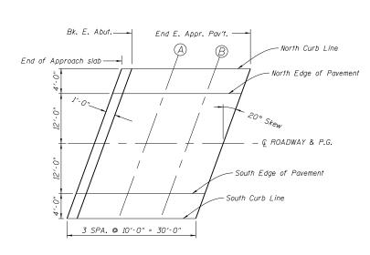
Top of slab elevations are after the Diamond Grinding of the Approach Slabs. Add 0.02' to the theoretical grade elevations for top of slab elevations prior to Diamond Grinding.
