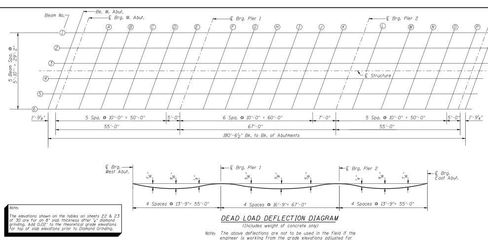
engineer is working from the grade elevations adjusted for Dead Load deflections as shown on sheets 22 & 23 of 29.
