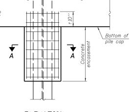
Welded wire fabric 6 x 6-W4.0 x W4.0 weighing 58#/100 sq. ft. Bend as required to fit into wall.
