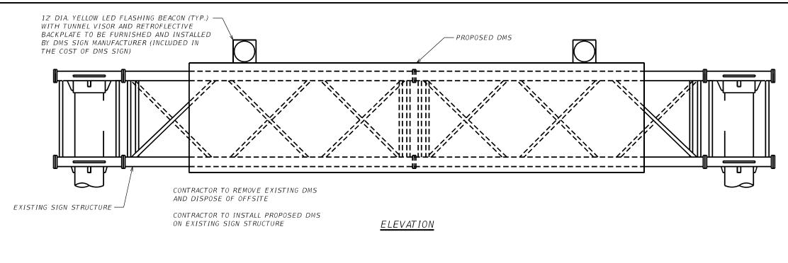
NOTE: THE CONTRACTOR SHALL SUBMIT COMPLETE ELECTRICAL DESIGN DETAILS AND CALCULATE SEALED BY AN ILLINOIS LICENSED ELECTRICAL AND STRUCTURAL ENGINEER TO THE RESIDENT ENGINEER FOR REVIEW AND APPROVAL PRIOR TO THE ORDERING OF ANY MATERIALS.
