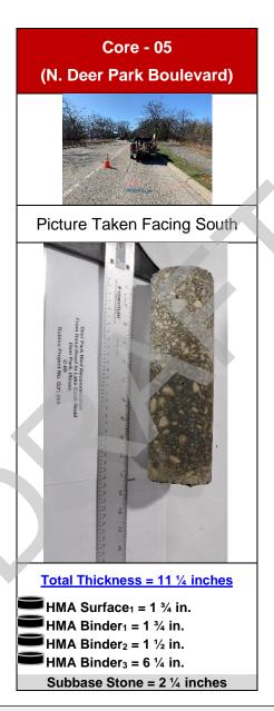
The referenced thicknesses are considered approximate. Commentary provided by Rubino is based on our observation in the laboratory; **Crack** = vertical through cross section; **Weathering** = rounded edges & degradation of asphalt and **Deterioration** = horizontal crack. Pavement and subbase type and thickness may vary between core locations. Any comments on the condition of the material are considered our opinion and should be verified by the design engineer.
