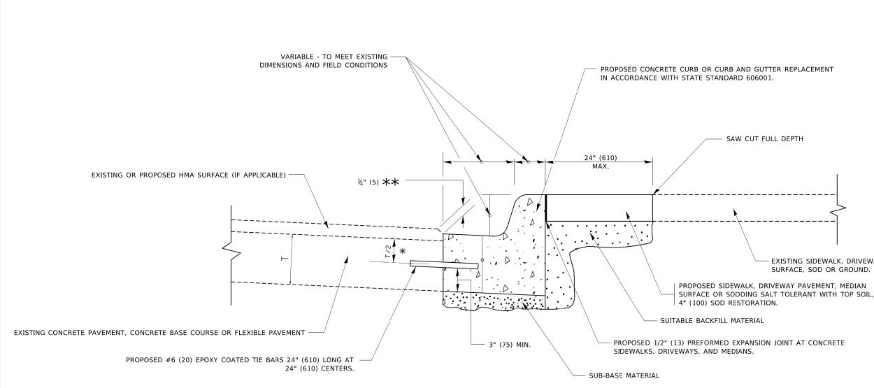
★ 3" (75) MINIMUM FROM TOP AND BOTTOM OF THE CONCRETE PAVEMENT OR BASE COURSE.
