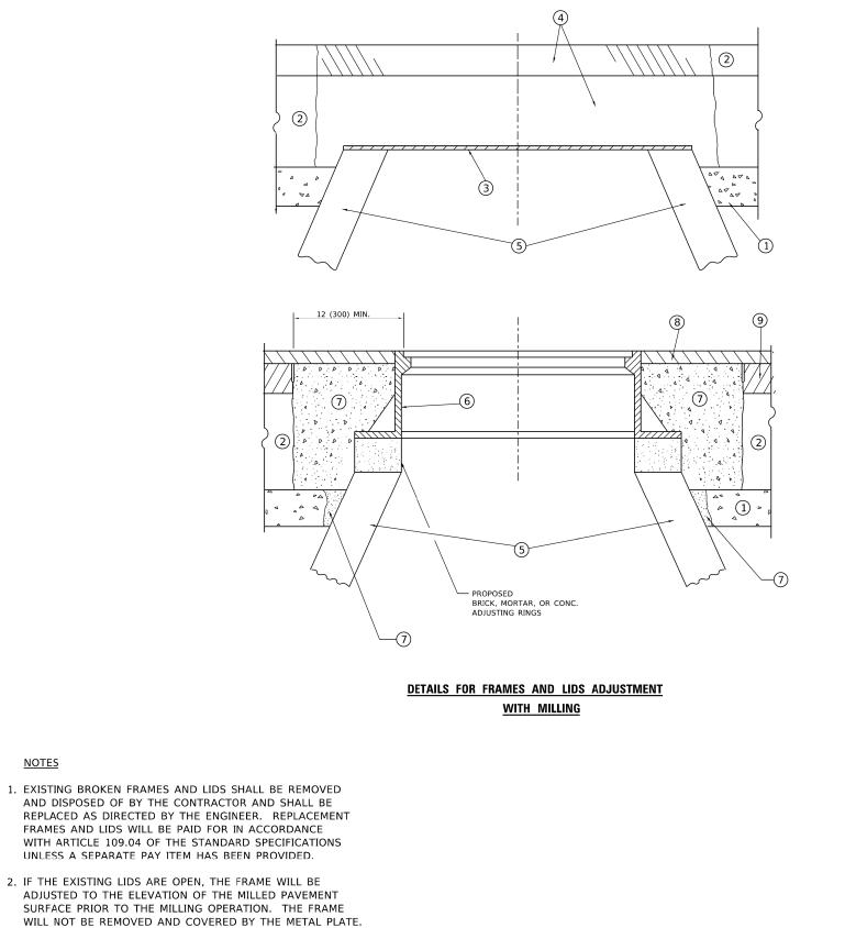
3. CITY OF CHICAGO CASTINGS ARE THE PROPERTY OF THE CITY AND THE CONTRACTOR SHALL NOTIFY THE CITY FOR REMOVAL AND DISPOSITION OF THE CASTINGS.
