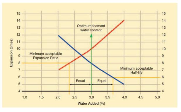
Repeat Steps 1 through 9 for two other bitumen temperatures normally 340  $^{\circ}$ F (170  $^{\circ}$ C) and 360  $^{\circ}$ F (180  $^{\circ}$ C). The temperature and optimum water addition that produces the best foam is then used in the mix design procedure described below.
