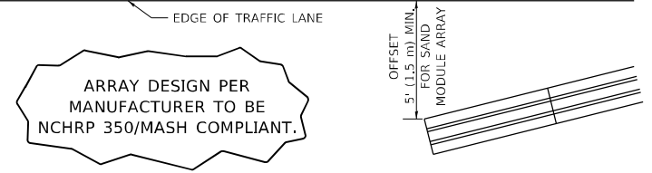
DETAIL "A" IMPACT ATTENUATOR, TEMPORARY (SEE NOTE 5)
