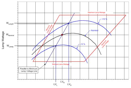
$\label{eq:ballast} \begin{aligned} & \text{Ballast Regulation} = \frac{W_{LampH} - W_{LampL}}{W_{LampN}} \times 100 \end{aligned}$
