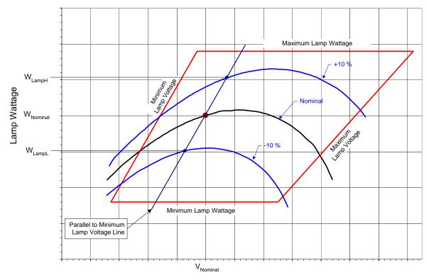
$$\label{eq:ballast} \text{Ballast Regulation} = \frac{W_{\textit{LampH}} - W_{\textit{LampL}}}{W_{\textit{LampN}}} \times 100$$
