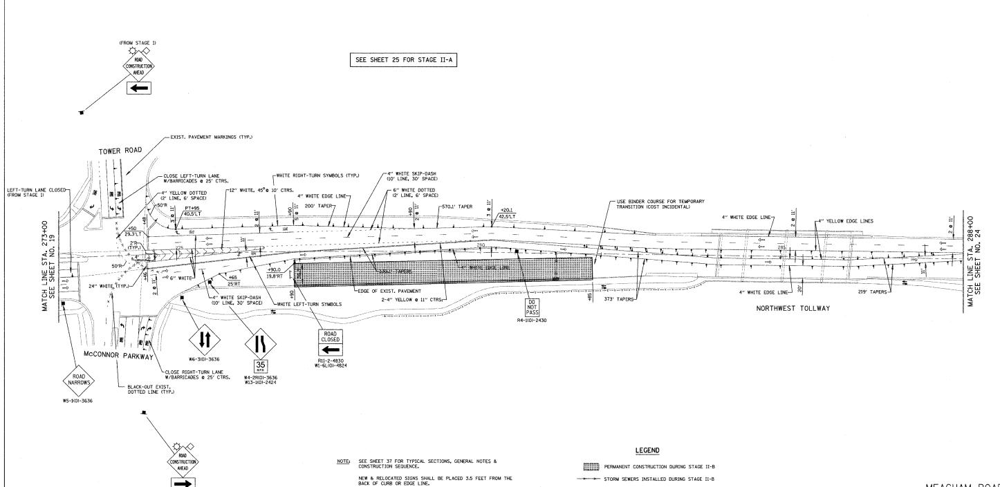
ALL PROPOSED PAVEMENT MARKINGS ON THIS SHEET SHALL BE "TEMPORARY PAVEMENT MARKINGS" IN ACCORDANCE WITH ARTICLE 703.05 OF THE "STANDARD SPECIFICATIONS".
